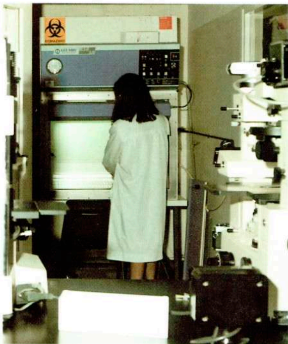
Shared areas in biomedical research. Laminar flow camera. Camara de fluxe laminar a recerca biomèdica.
